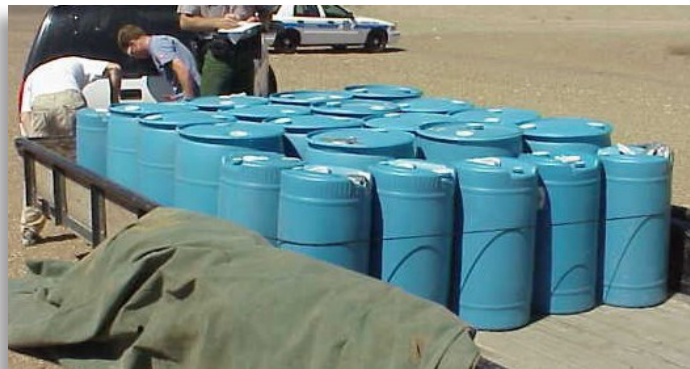
These polyethylene drums were found to be full of gasoline, a Class IB flammable liquid. Their capacity for Class IB liquids exceeds that permitted by the model codes.
